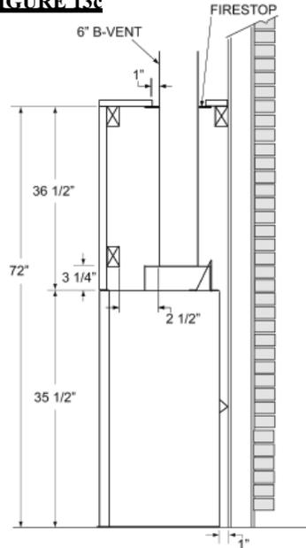
The fireplace requires a minimum enclosure height of 72". For temperature requirements, the enclosure space around and above the fireplace must be left unobstructed.
