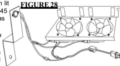
Attach and secure the sensor assembly bracket to the securing stud located next to the receptacle/junction box at the bottom left of the unit using the lock washer and wing nut. Ensure that the thermidisc touches the firebox wall.
