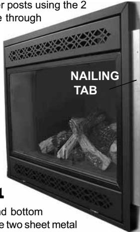
Drill through the centre of the top and bottom slots in the nailing tab. Secure using the two sheet metal screws supplied. This allows the nailing tab to slide back and forth for desired framing. Figure 12 b.
