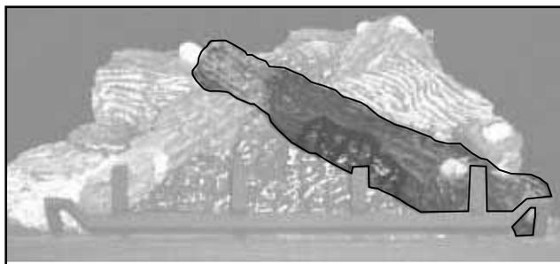
5. Place the bottom of the right crossover log (W135-0302) onto the stud on the right side of the log support. The top of the log should rest in the pocket on the left crossover log (W135-0300).
