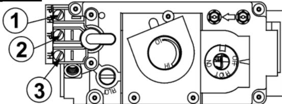
Do not connect either the wall switch, thermostat or gas valve directly to 110 volt electricity.
