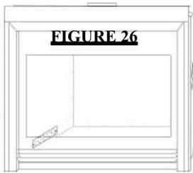
Position the vibration reducing pad into the clip and onto the threaded stud at the other end, piercing a hole into the pad. The fan assembly must be able to be positioned entirely onto the pad.
