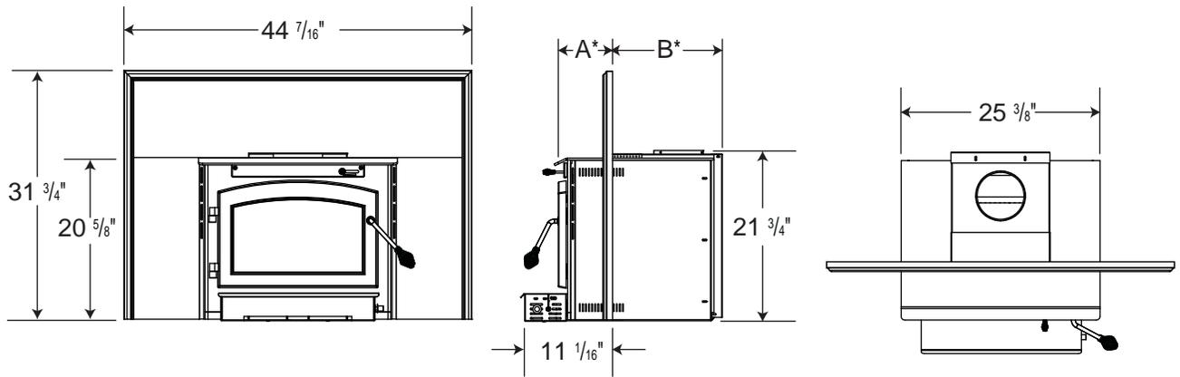
\* A and B are adjustable in  $\frac{3}{8}$ " increments (see min max below).
