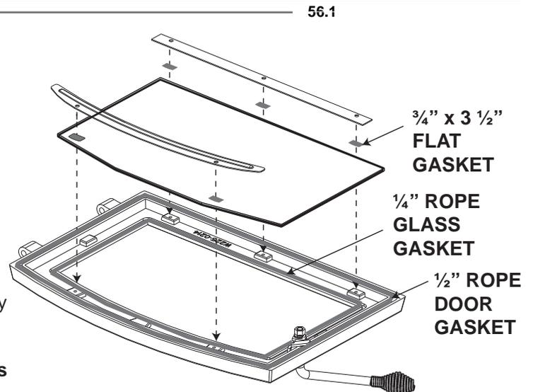
**NOTE:** For replacement glass, size, thickness and specifications see "REPLACEMENTS" section.
